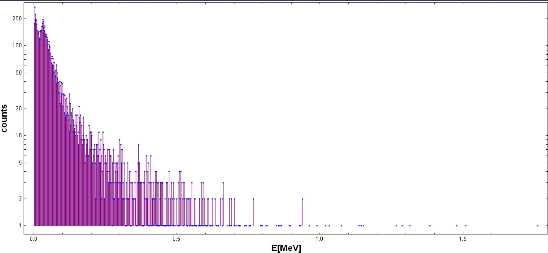
Spectrum of deposited energies of bremsstrahlung radiation
