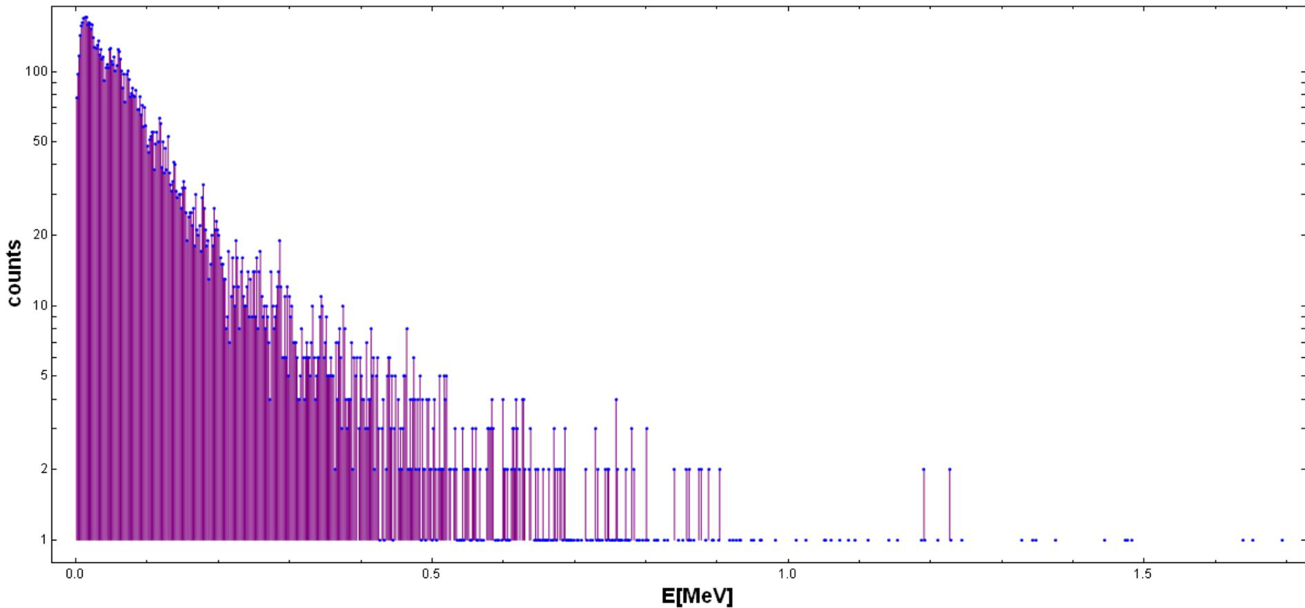
Spectrum of deposited energies of bremsstrahlung radiation
