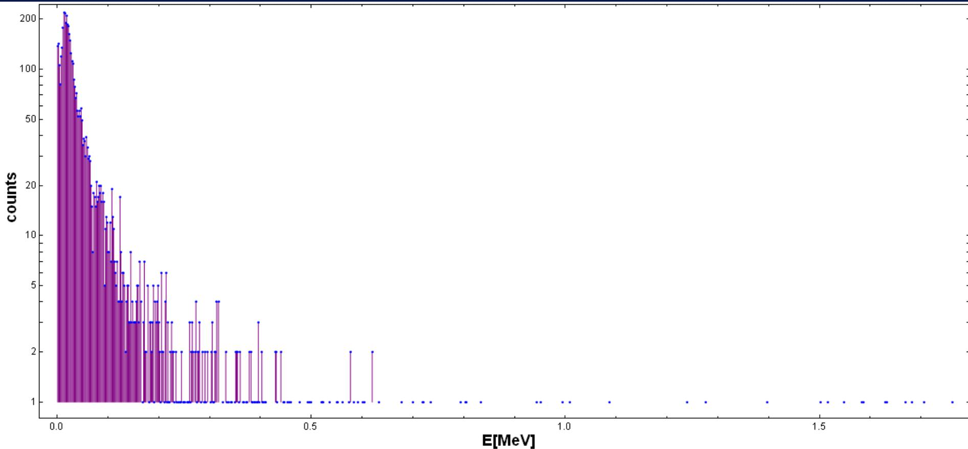
Spectrum of deposited energies of bremsstrahlung radiation
