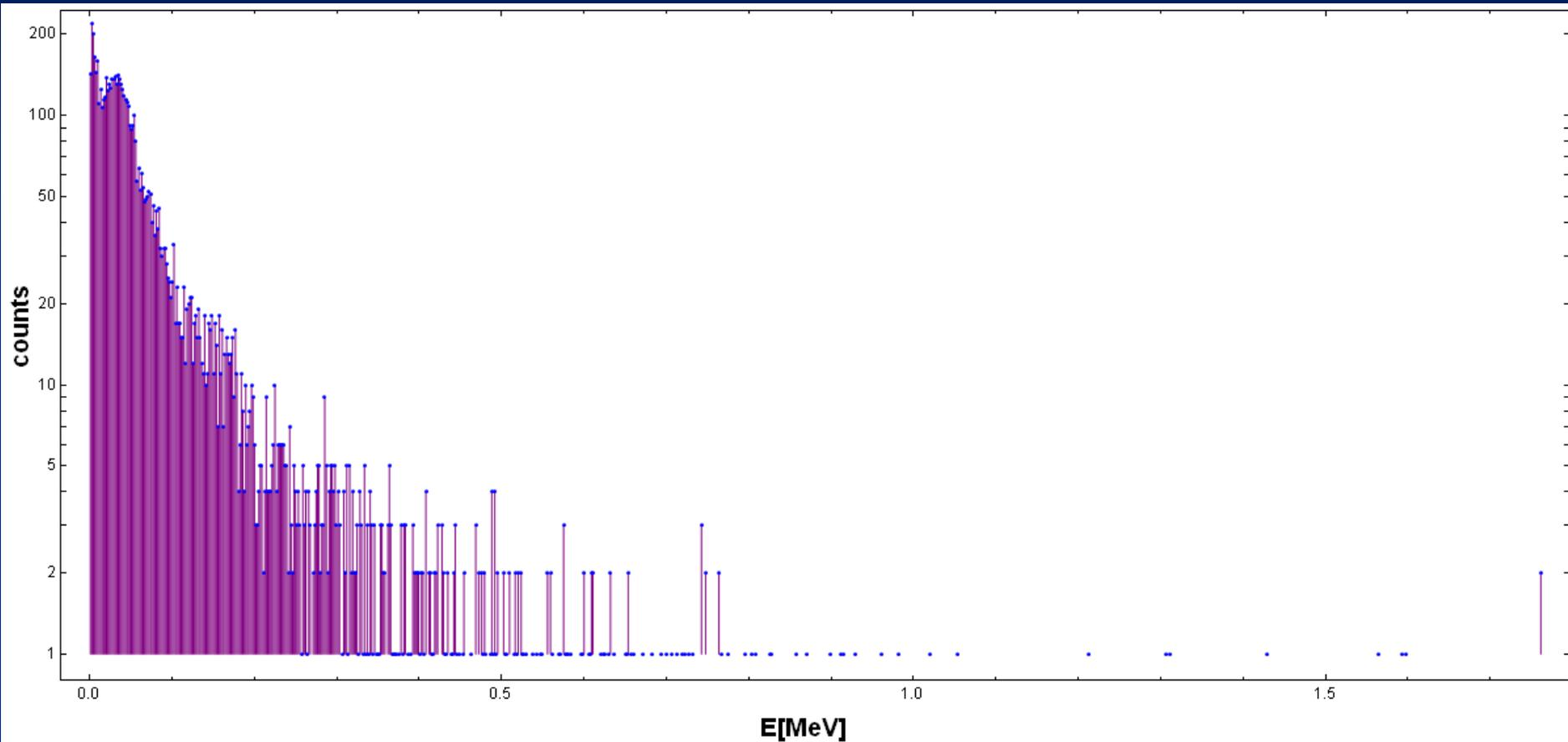
Spectrum of deposited energies of bremsstrahlung radiation
