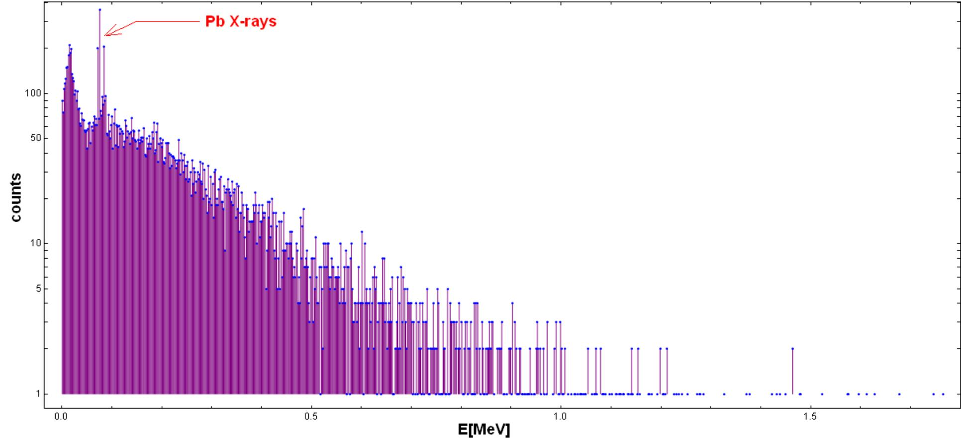
Spectrum of deposited energies of bremsstrahlung events in water cylinder
